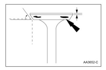
2. Inspect for abnormalities on the valve face and seat. Install a new cylinder head assembly if abnormalities are found.
